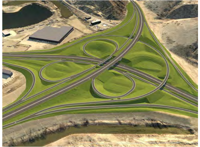
Example Highway 14/169 turbine interchange developed with InfraWorks
