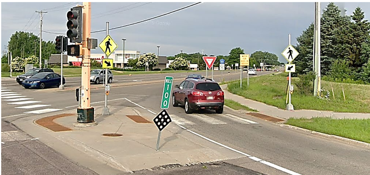
Illustration of channelized right-turn best practice (top). Example of LED pedestrian warning signage at a channelized right-turn along TH 13 in Burnsville (bottom).
